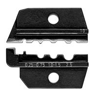
Application: non-insulated tubular cable lugs and crimp terminals in accordance with DIN 46237 and non-insulated butt and crimp connectors in accordance with DIN 46341 0.75 / 1.5 / 2.5 mm²
