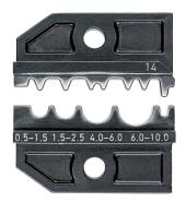
Application: for non-insulated crimp terminals, tube and compression cable lugs in accordance with DIN 46234 and DIN 46235 and non-insulated crimp, butt and press connectors in accordance with DIN 46341 and DIN 46267 0.5-10 mm<sup>2</sup>
